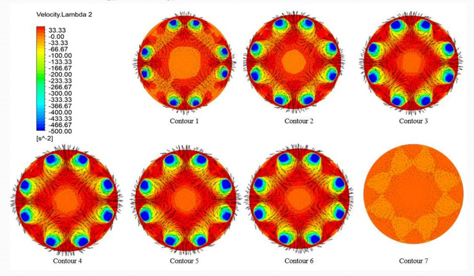
Velocity profiles of case 1 for  $\text{Re}_{hw} = 8000 - \text{Re}_{cw} = 2000$ .
