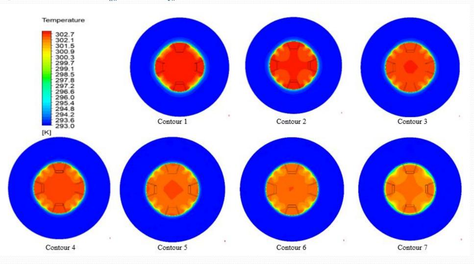
Temperature profiles of case 1 for  $\text{Re}_{hw} = 8000 - \text{Re}_{cw} = 2000$ .
