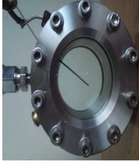
Figure 2: Viscosity/solubility/miscibility cell (left) and miscibility/solubility cell (right)
