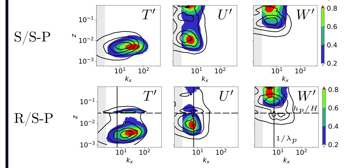
Spectral density as a function of the altitude z. Colors: periodic case; Lines: cavity; Shaded area: unreachable k in the fluid layer.
