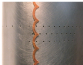
T2 Cascade Local roughness on suction side
