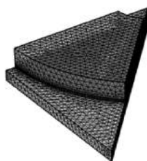
Figure 6: Example of the mesh generated by the COMSOL software for Extra Fine selection.
