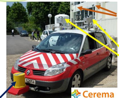
Radiometer ThermoRoute II (CEREMA)
