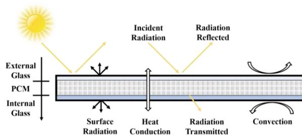
Figure 2.1: *Physical model of PCM glazing unit*
