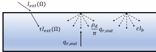
Figure 2.2: Radiative intensity entering glazing unit along the  $\Omega$  direction
