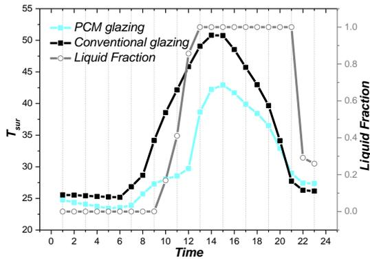
Figure 3.3: Comparison between PCM glazing and conventional glazing by  $T_{sur}$
