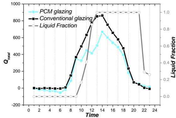
Figure 3.4: Comparison between PCM glazing and conventional glazing by  $Q_{total}$
