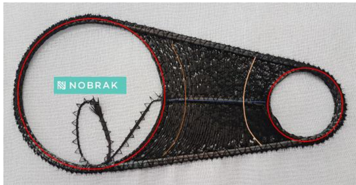
Fig. 1 - TFP preform made of commingled yarns. The red and yellow lines show fiber orientation.
