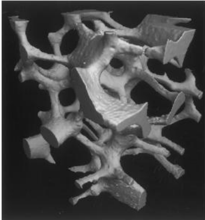
Fig. 3. Synchrotron tomographic image of AA6101 Al foam at a resolution of 23 \mu\text{m} . The structure is predominately open-celled. The rough surface of cell walls (edges) is a result of the casting process.
