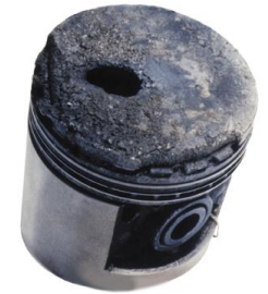
Piston damage by long-term knock (Lawrence Livermore National Laboratory)
