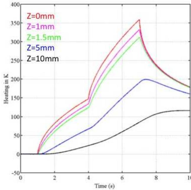
Figure 3b - Corresponding temperature responses for several positions
