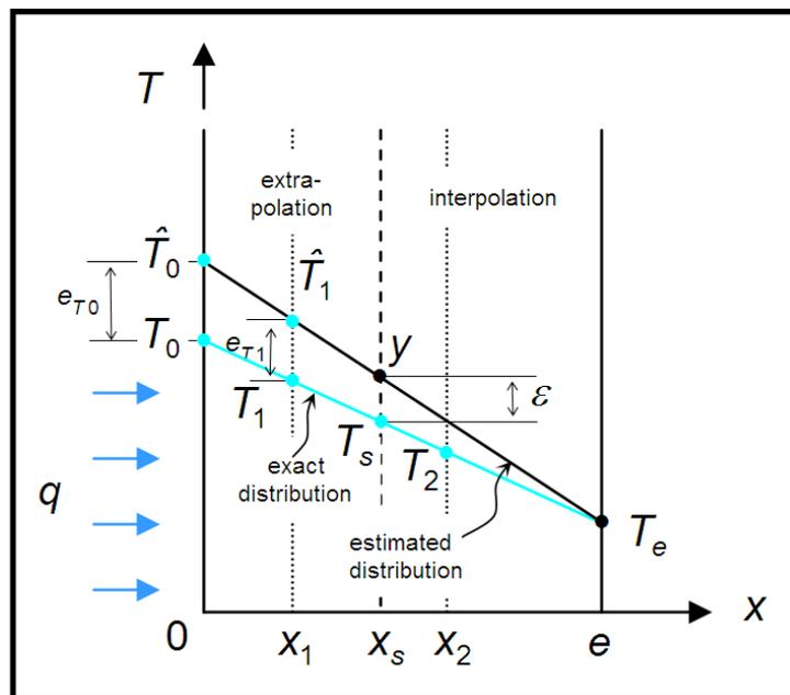
**Figure 2a** – Estimation of temperature/flux in a wall
