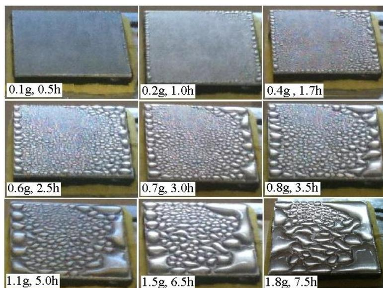
Figure 4. Photographs of the flat plate covered with condensation at different instants of a trial.
