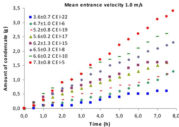
Figure 3. Amount of condensate as a function of time for different average temperature differences ( $\Delta T_c$ ) under a 1.0 m/s mean entrance velocity.
