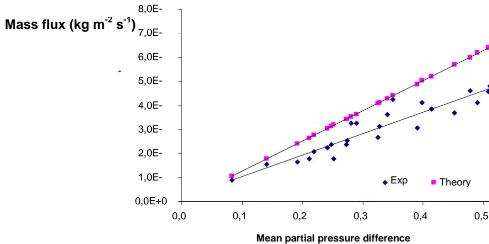
Figure 5. Mass flux for a mean entrance velocity of 1.0 m/s as a function of the mean partial pressure difference.
