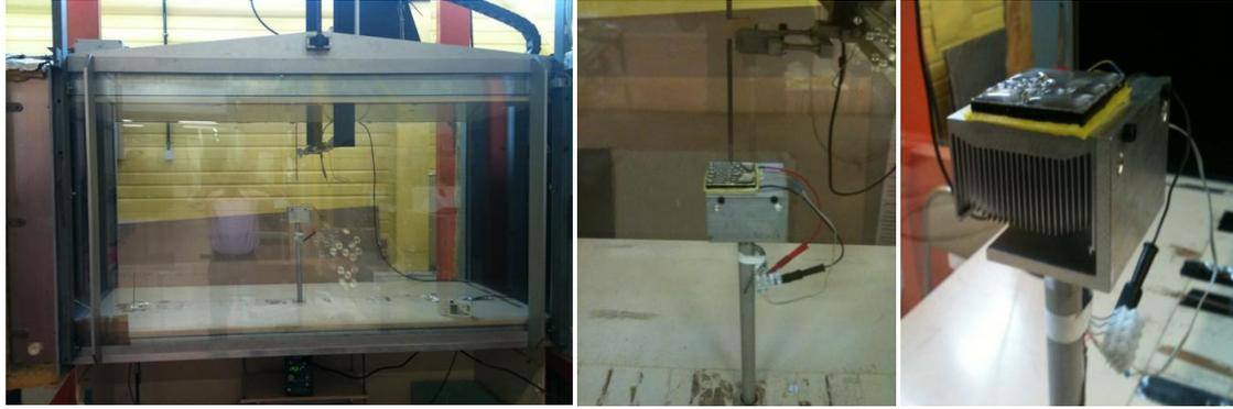
Figure 1. Photograph of the test chamber and close look at the condensing unit in the presence of drops on top of the active surface.
